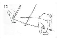
Connect the horizontal bottom pipes to the wall pipes. Note: twist to lock in place.
