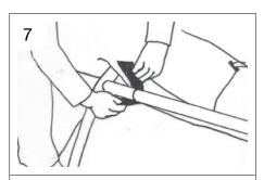
Attach the roof cover to the roof frame with the black Velcro straps.
