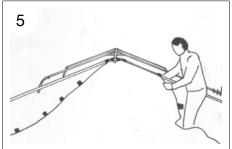
Attach the front and back gable covers to the roof frame. Use the black velcro straps, starting from the apex.
