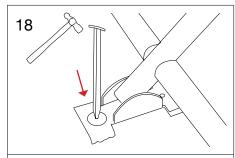
IMPORTANT: Anchor the base plates with V-pegs
