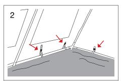
Starting from one doorway, fix the groundsheet to the side walls by fixing the toggles to the rings.
