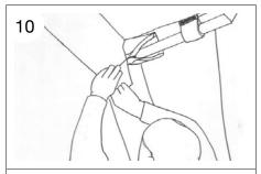
Seal the cover overlaps in the corners and at the apex with Velcro and close the cuffs
