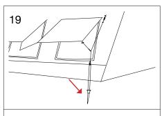
IMPORTANT: Attach the guy lines and anchor with V-pegs
