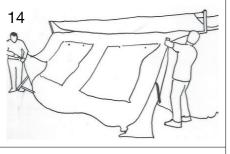
Pull down the side walls of the roof cover.
