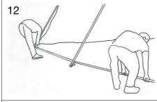
Connect the horizontal bottom pipes to the wall pipes. Note: twist to lock in place.
