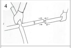
Assemble the other side of the roof frame.
