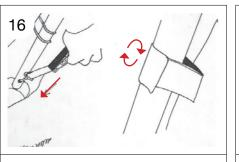
Finish fixing gable covers to wall poles. Fix the straps with hook at the bottom corners to the wall pipes, then complete the Velcro straps.
