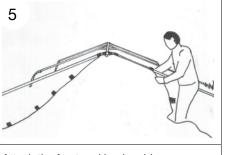
Attach the front and back gable covers to the roof frame. Use the black velcro straps, starting from the apex.
