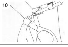
Seal the cover overlaps in the corners and at the apex with Velcro and close the cuffs
