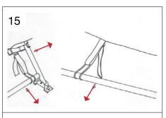
Use the hooks to attach to the bottom pipes and tighten
